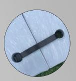
**Single Steel Joiner** (12mm round bar) – the most robust option but requires the mats to be lifted through 90 degrees to install. Available in uncoated or zinc plated finish
