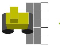
2: Maximum of two further rows of CellPave™ AP tiles added and rolled in, leaving last row unrolled
